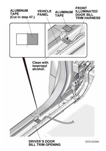
53. Secure the front illuminated door sill trim harness to the vehicle panel with one piece of aluminum tape cut in step 47.
