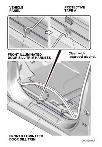
24. Install the protective clip to the protective tape A on the vehicle panel.
