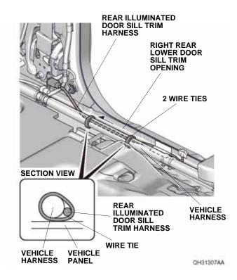
68. Plug the door sill trim harness 2-pin connector into the rear illuminated door sill trim harness 2-pin connector, and secure the 2-pin connectors and door sill trim harness to the vehicle harness with three wire ties as shown.
