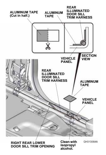
66. Using scissors, cut one aluminum tape in half, and secure the rear illuminated door sill trim harness to the vehicle panel with one piece of aluminum tape as shown.
