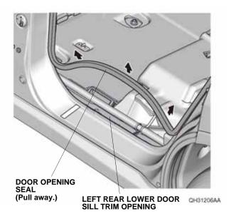
28. Using an alcohol wipe, thoroughly clean the vehicle panel where the rear illuminated door sill trim will attach.
