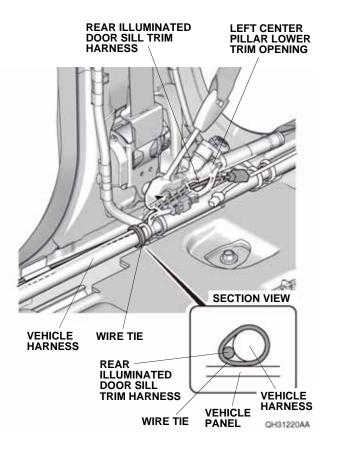
49. Plug the door sill trim harness 2-pin connector into the rear illuminated door sill trim harness 2-pin connector.
