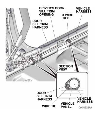
52. Using isopropyl alcohol on a shop towel, thoroughly clean the vehicle panel where the aluminum tape will attach.
