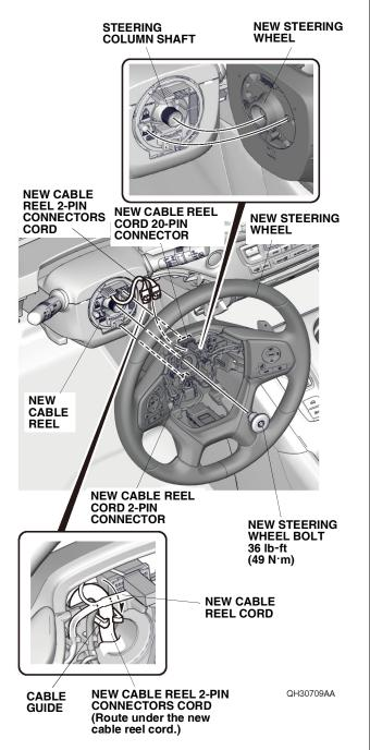
39. Install the new steering wheel bolt. Torque the new steering wheel bolt to 36 lb-ft (49 N·m). Tighten at the specified torque within 5 minutes.
