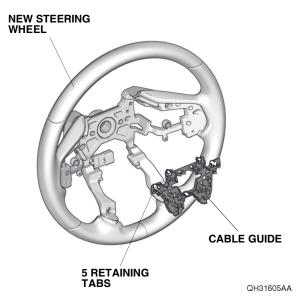
30. Install the new cable reel cord to the cable guide with one washer-screw removed in step 27. Plug the new cable reel cord 4-pin connector into the new steering wheel 4-pin connector, and secure the new cable reel cord to the cable guide.
