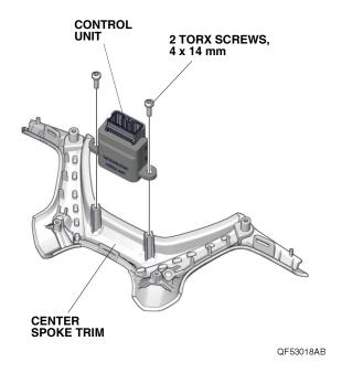
33. Plug the new cable reel cord 14-pin connector into the control unit, and install the center spoke trim to the new steering wheel with two self-tapping screws removed in step 25.
