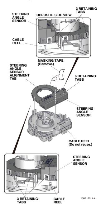
19. Install the steering angle sensor to the new cable reel with six retaining tabs.
