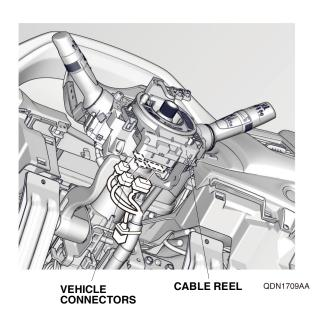
17. To prevent turning from the cable reel, apply masking tape to the cable reel. Remove the cable reel.
