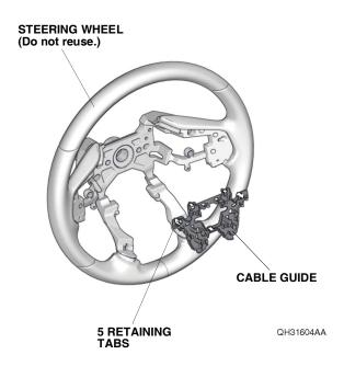
29. Install the cable guide on the new steering wheel with five retaining tabs.
