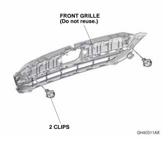
11. Install the two clips to the new front grille.
