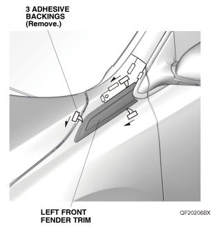
6. Using a rubber roller, apply firm pressure against the left front fender trim and roll from one end to the other. Apply firm pressure, especially at the ends.
