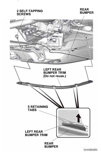
11. Install the new left rear bumper trim to the rear bumper with two self-tapping screws and five retaining tabs.
