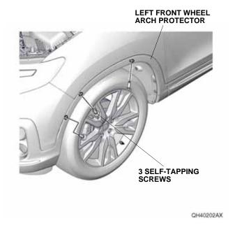
B. Remove the left front wheel arch protector.
