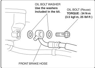
8. Remove the cap from the supplied front brake hose.
