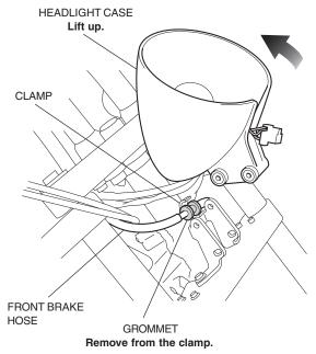
6. Disengage the front brake hose grommet from the clamp as shown.
