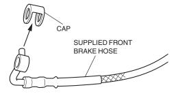
9. Install the supplied front brake hose in the reverse order of the original hose removal.
