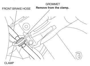
7. Remove the oil bolt and disconnect the front brake hose.
