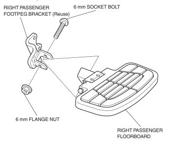
4. Install the right passenger floorboard as shown.
