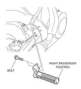
2. Remove the right passenger footpeg from the bracket.
