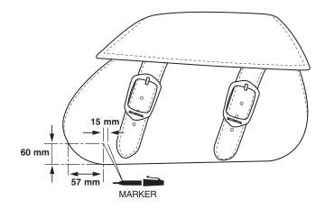
6. Using an electric drill and drill bit, drill a 9 mm and 4 mm hole through each of the two marks you just made as shown.
