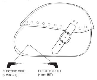
7. Install the reflex reflectors on the right saddlebag as shown.
