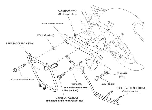
4. Torque all 10 mm bolts to the specification in the torque chart.
