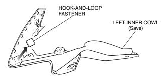
5. Attach the hook-and-loop fasteners to the accessory inner cowls in the position shown.
