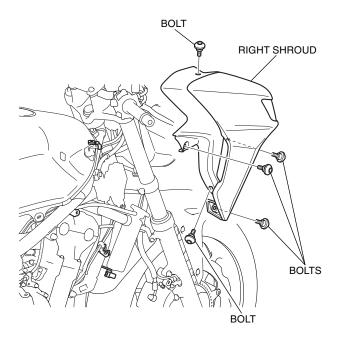
3. Remove the existing inner cowls as shown.
