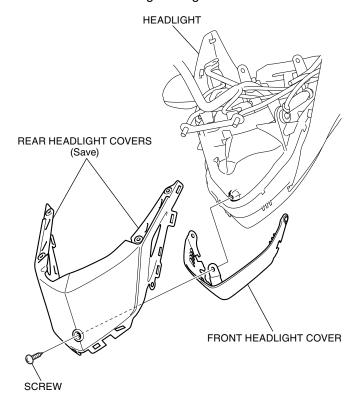
10. Assemble the accessory rear headlight covers as shown.
