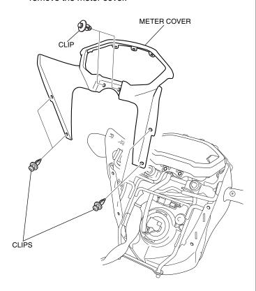
8. Refer to the Service Manual for the motorcycle, remove the meter visor.
