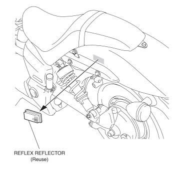
2. Remove the double-sided adhesive tape from the reflex reflector you just removed.
