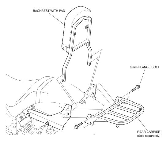
9. Tighten the parts that you installed loosely.
