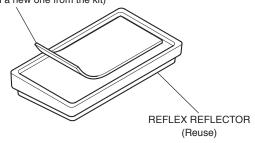
3. Using an isopropyl alcohol solution, thoroughly clean the left rear side of the rear fender where the reflector will be attached. Attach the reflex reflector to the rear fender in the area shown.
