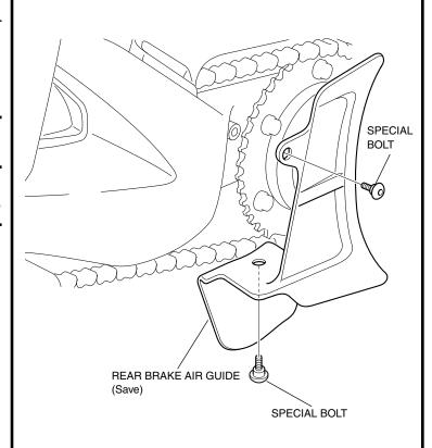
2. Apply thread lock to the mounting bolts as shown.
