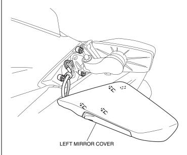
4. Remove the left turn signal light harness as shown.
