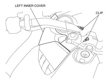
2. Remove the left inner cover, and then disconnect the negative (-) battery cable.
