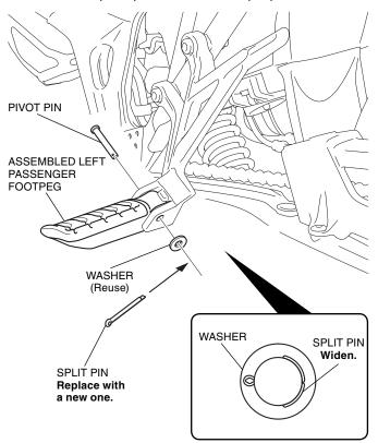
10. Check that the left comfort passenger footpeg is fixed at each position by moving it as shown.
