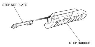
4. Install the assembled step rubber to the left footpeg arm as shown.
