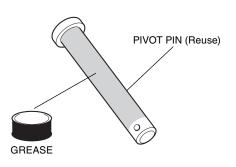
9. Install the pivot pin, washer, and split pin as shown.
