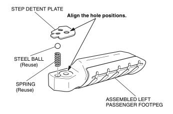
7. Install the assembled left passenger footpeg while holding down the step detent plate.
