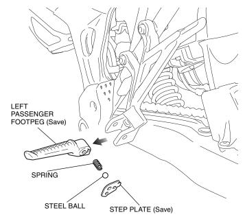
3. Assemble the step set plate and step rubber as shown.
