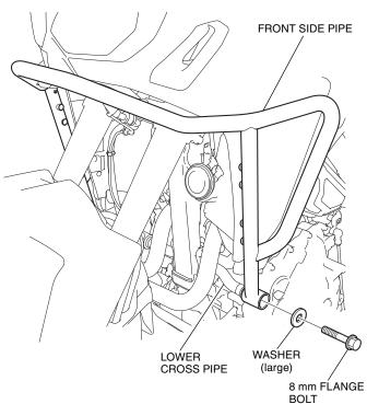
13. Loosely install the front side pipe as shown.
