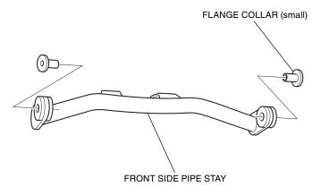
3. Loosely install the assembled front side pipe stay as shown.
