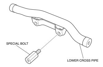
5. Pass the assembled lower cross pipe as shown.
