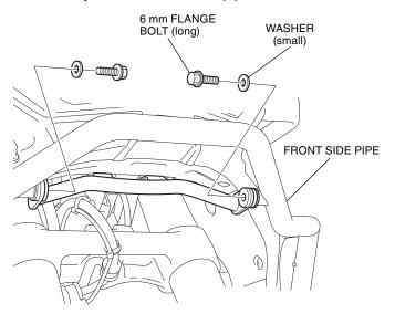
14. Securely tighten the 6 mm screws, and then tighten the 6 mm flange bolts.
