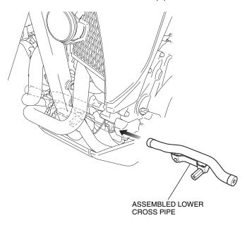
6. Install the special bolt as shown.
