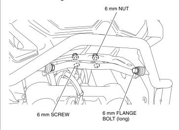
15. Securely tighten the 8 mm flange bolts, then tighten the 6 mm flange bolts.
