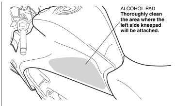
2. Attach the left side kneepad in the position shown to follow the contours of the tank. Repeat this step on the right side.
