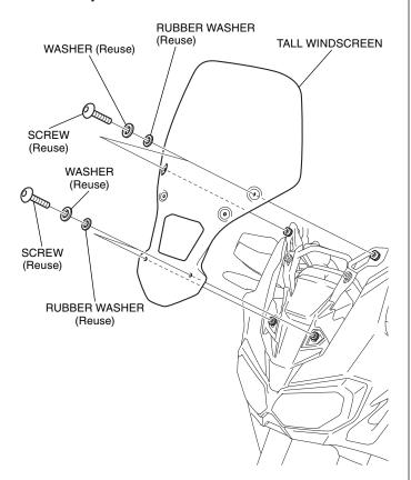
5. Loosely install the 5 mm screws as shown.
