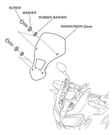
2. Remove the well nuts as shown.
