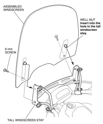
14. Align the windscreen assembly in accordance with the dimensions shown and check that the windscreen is positioned equally on both sides, then tighten the screws, bolts, and nuts to the specifications in the Torque Chart.
