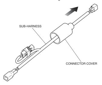
19. Remove the meter connector as shown.
