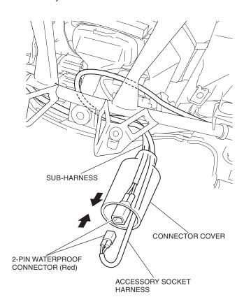
29. Secure the sub-harness and accessory socket harness using the wire tie as shown.
