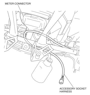
28. Route the accessory socket harness through the connector cover as shown, and connect the accessory socket harness to the sub-harness.
