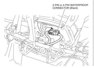
21. Remove the connector as shown.
