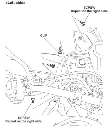
Remove the left fuel tank side cover as shown.
