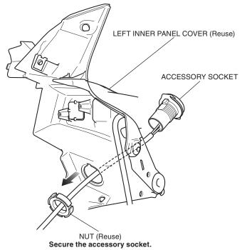
Route the accessory socket harness as shown, and install the left inner panel cover in the reverse order of removal.
