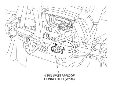
22. Remove the dummy connector as shown.
