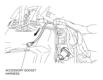
17. Wind the electrical tape around the sub-harness as shown.
