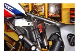
The dispenser can be held using the small dispenser plate and clip, secured by the rear sprocket guard bolt. The tip of the injector should lightly touch the face of the sprocket, with the slash cut facing outwards. The delivery tubing can be routed *inside* the swing arm to the rear of the suspension unit, and up to the RMV on the sub frame.
